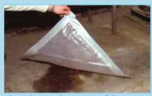
The poly test determines if drylooking masonry is passing water. Left overnight, a plastic sheet will cause misleadingly dry-looking concrete to dampen visibly.
